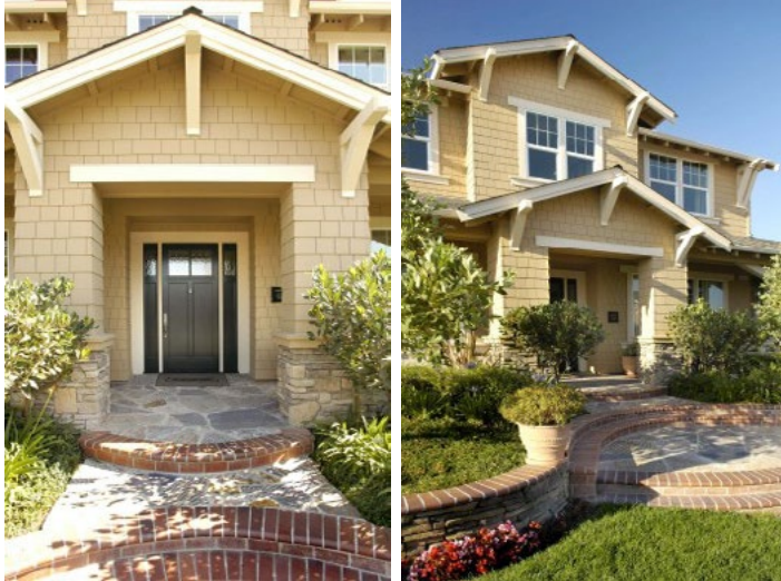
Wood and shingle siding, broad porches, and exposed rafter tails all spell the Craftsman theme
