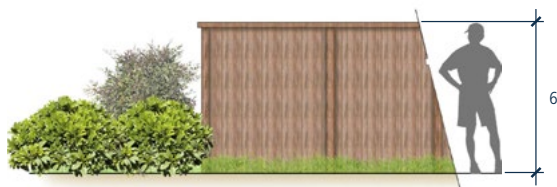
SIDEYARD WOOD/VINYL FENCE SCALE: N.T.S.
