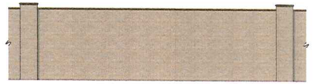
● 6' Ht. Slump Block Wall with Slump Block Cap with Pilasters at Property Lines set on 24" berm. Property walls at lots to be 5' Slump Stone with Slump Stone Cap
