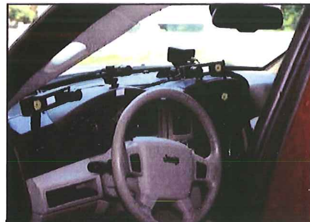
For the field study, a Jeep Cherokee was outfitted with three eye-tracking cameras on the dashboard
