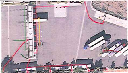
PHOTO PROVIDED BY CLIENT GREEN = STORM DRAIN/SEWER RED = LIGHTING/ELECTRIC PINK = PRODUCT LINES/VENT PIPES ORANGE = CONDUIT TO EMERGENCY SHUTOFF PEDESTALS
