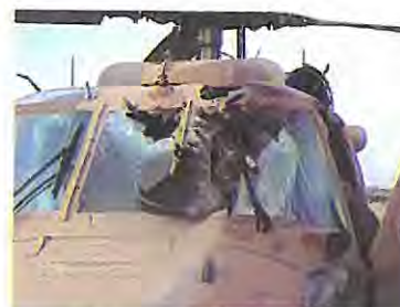
A Sikorsky UH-60 Black Hawk after a collision with a common crane (bird), and resulting failure of the windshield.
