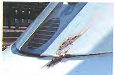
An ICE 3 high speed train after hitting a bird
