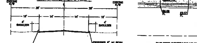
BARNETT ROAD (NORTH) TYPICAL SECTION NORTH OF MCLAUGHLIN ROAD SCALE: HORIZ. 1" = 10' VERT. 1" = 10'
