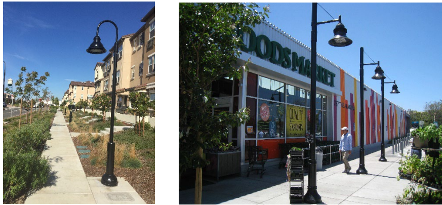
Figure 3.01.11-1. Shielded Light Fixtures
