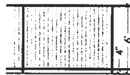
TUBE FENCE 2" SQUARE TUBE POST @ 8' O.C. 1 1/2" TUBE TOPS BOTTOM RAILING 1" SQUARE PICKLE @ 4' O.C.
