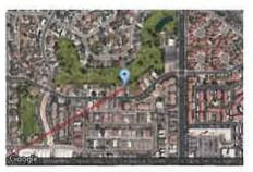
**Point** Latitude Longitude **Ground elevation** Height above ground Total elevation ft ft ft deg deg Threshold 33.920392 -117.263515 1583.43 1400.07 2983.50 2-mile point 33.905428 -117.293362 1610.68 1372.82 2983.50
