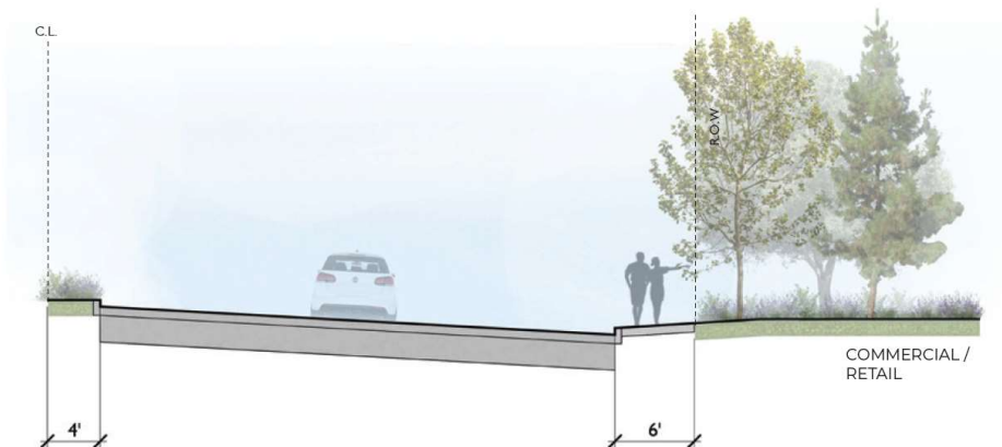
Figure 2-8: Rubidoux Boulevard Cross Section Arterial Highway
