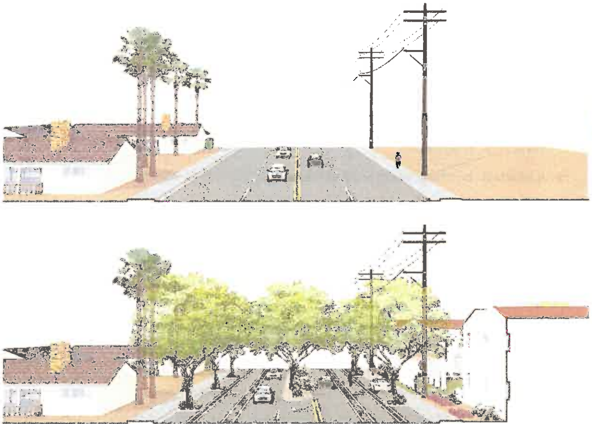
Example of a complete street transformation along Avenue 44 (existing street above, complete street below).
