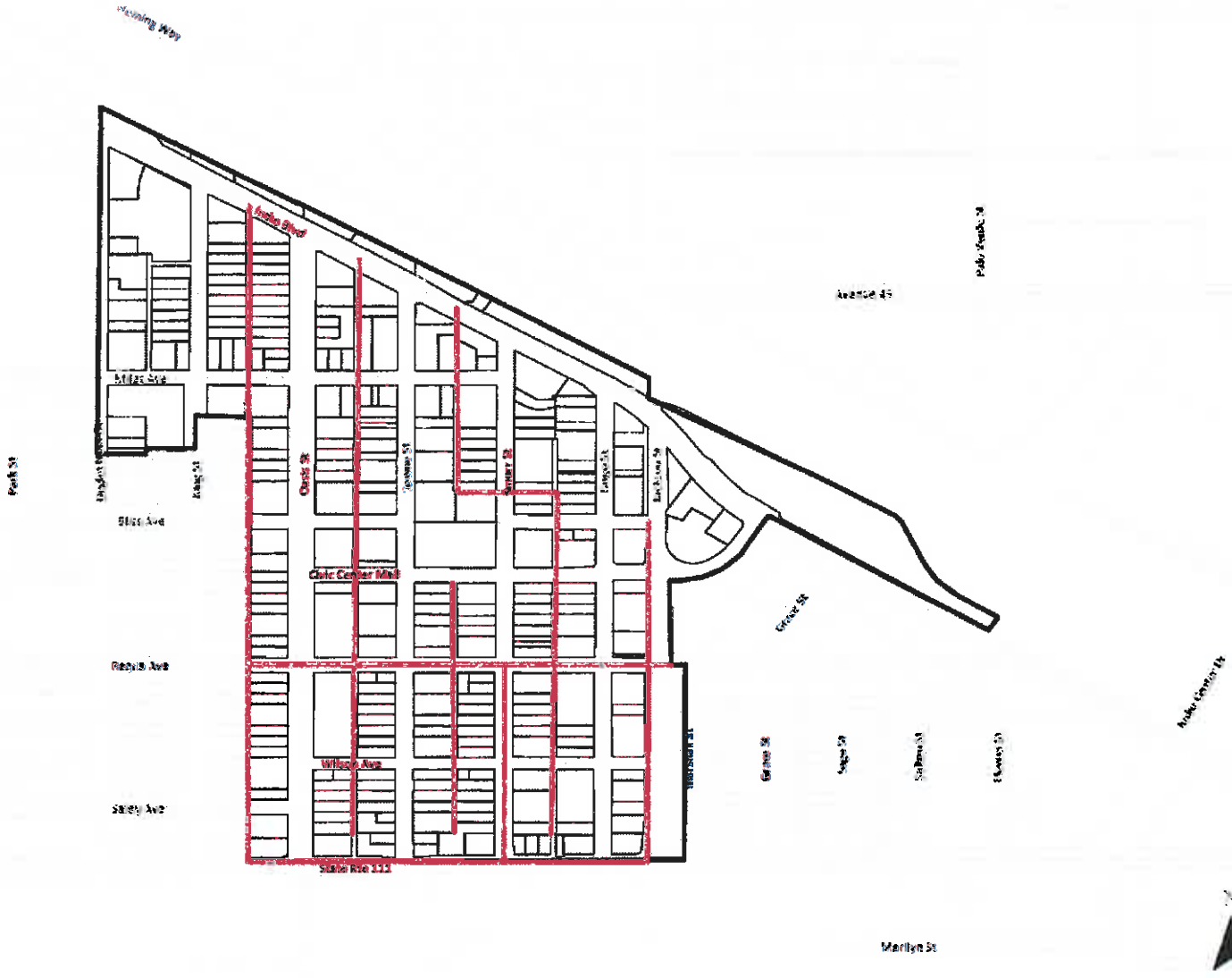
Figure 3-3 Existing Wastewater Lines
