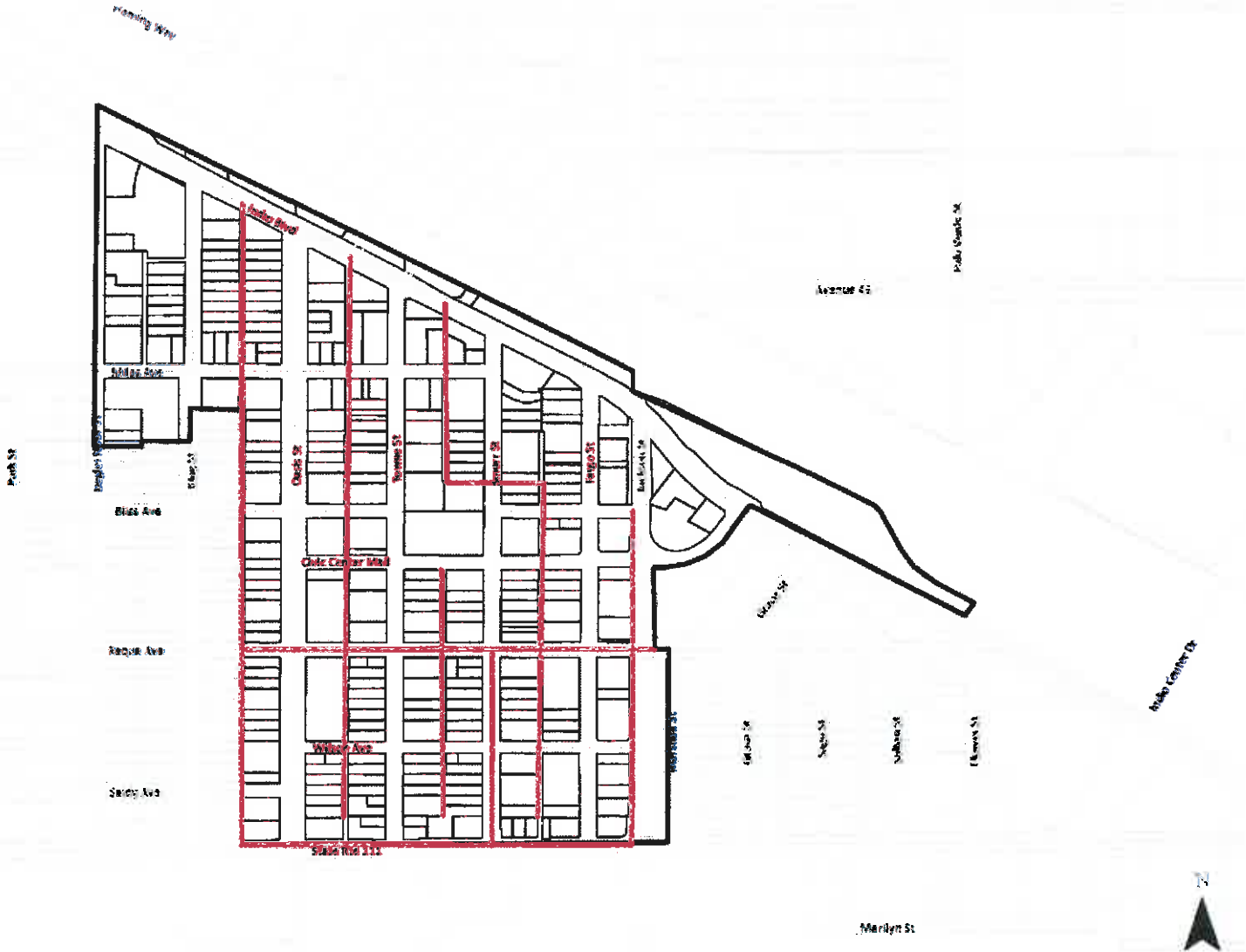
Figure 5-4 Existing Wastewater Lines
