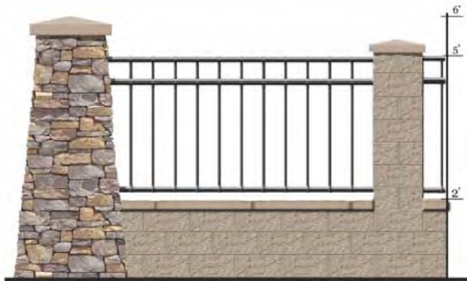
Split Wall/View Fence 2' Split Face Block With Wall Cap 3' Tubular Stainless Steel View Fence Battered Stone Veneer Pilaster With Concrete Cap in Accent Areas
