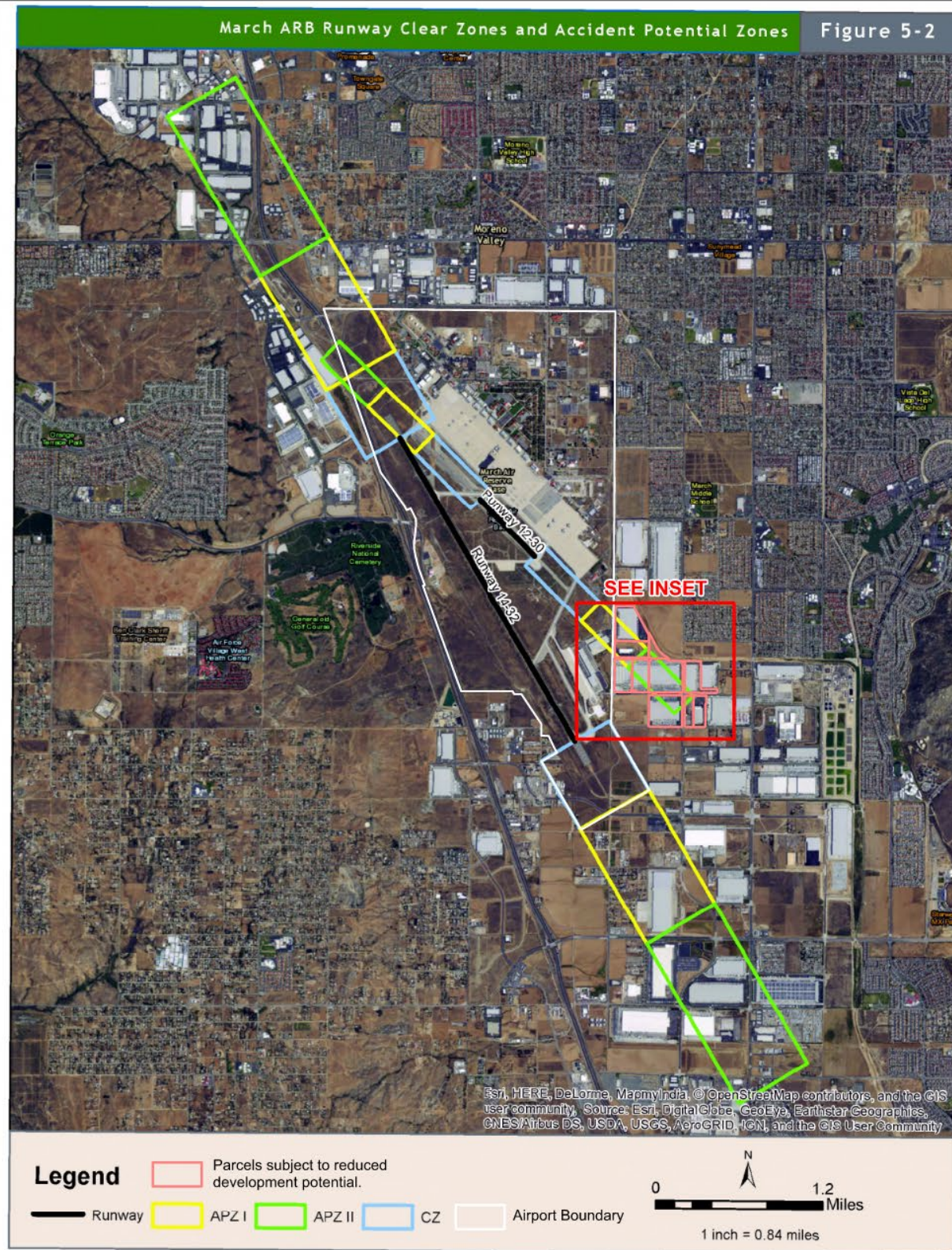
Exhibit 1: Exhibit MA-1B from the ALUCP Amendment showing parcels affected by March Air Reserve Base/Inland Port Airport Runway Clear Zones and Accident Potential Zones
