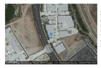
Name: PV Array 1 Axis tracking: Fixed (no rotation) Tilt: 10.0 deg Orientation: 180.0 deg Rated power: -Panel material: Smooth glass with AR coating Vary reflectivity with sun position? Yes Correlate slope error with surface type? Yes Slope error: Correlate with material
